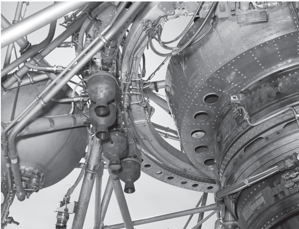
Two clusters of four rockets, designed to arrest the vehicle's descent, were attached to the LLRV's gimbal frame. These were later eliminated after tests determined they were unnecessary.
