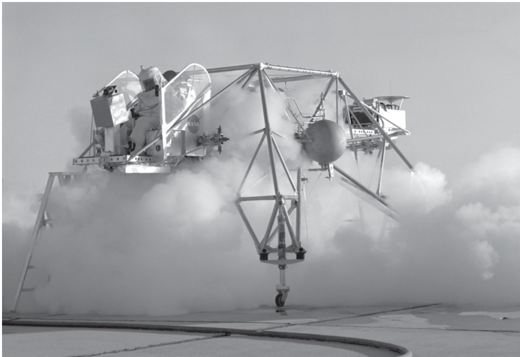
Shrouded in steam, the LLRV fires its lift-engines, located around the jet engine’s gimbal ring. The individual in the cockpit, like the ground crew, wears a protective suit against the possibility of being burned by hydrogen-peroxide droplets. (EC-64-447)
