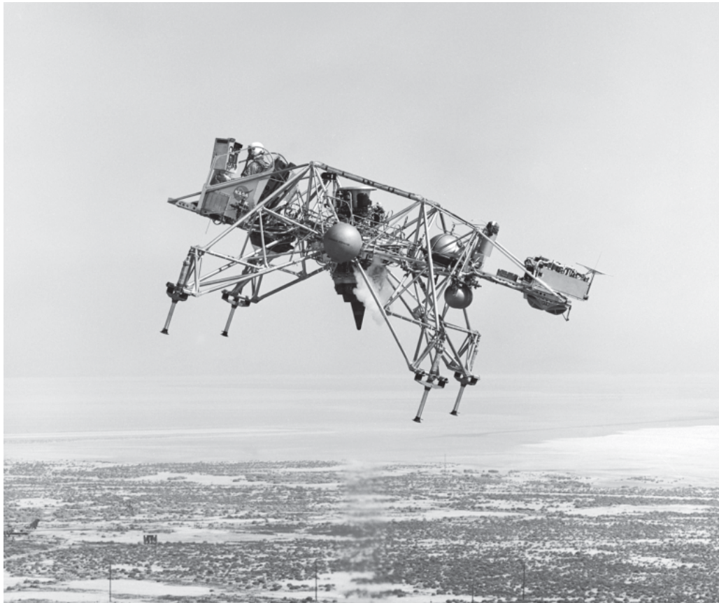
LLRV no. 1 in lunar simulation mode. The center-mounted jet engine is perpendicular to the Earth despite the LLRV's tilt angle. The jet engine supported 5/6 of the LLRV's weight, effectively simulating lunar gravity. The puff of steam aft of the jet engine indicates the rear lift rockets are firing to correct the tilt angle. (E-14570)
