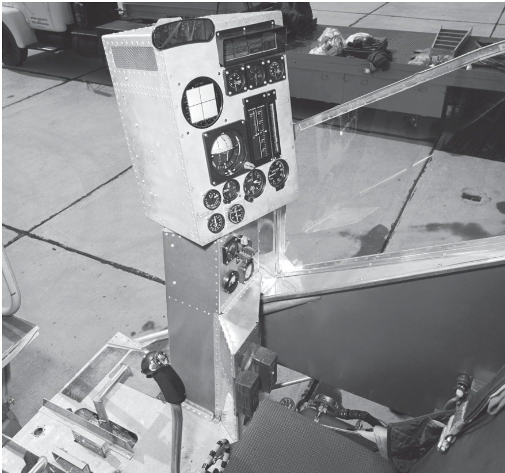
During the holiday break between 1964 and 1965 the crew took the opportunity to perform a number of modifications to the LLRV. They replaced the castering wheels on the vehicle's legs with dish-like footpads, and moved the pilot's instrument console from the center to the right side of the cockpit. (E-14317)
