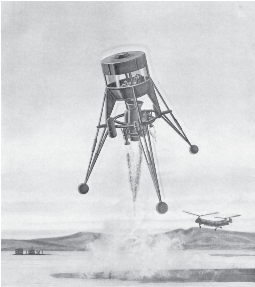
An artist's conception of the free-flight lunar landing simulator. During the first stages of planning, designers positioned the pilot directly above the jet engine intake to simplify center-of-gravity issues, but this led to distortion of the engine's intake flow. (ECN-8227)
